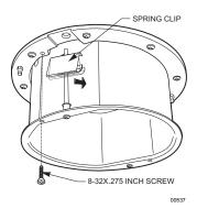
c. Compress the spring clips on the back box and push it through the hole until the clips spring back. Tighten the screws until you hear a clicking noise. Insert the two 8-32 x .275-inch screws to secure the back box to the mounting ring.
